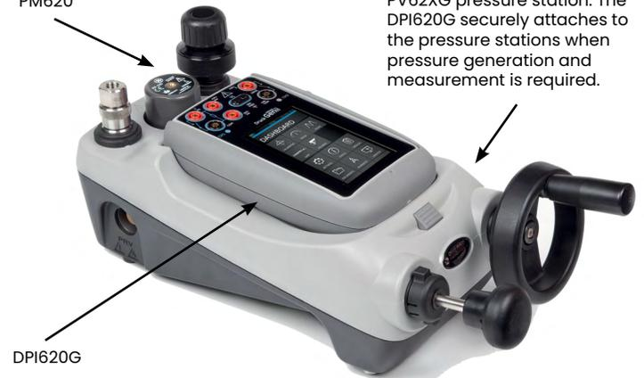
PV62XG pressure station. The DPI620G securely attaches to the pressure stations when pressure generation and measurement is required.
